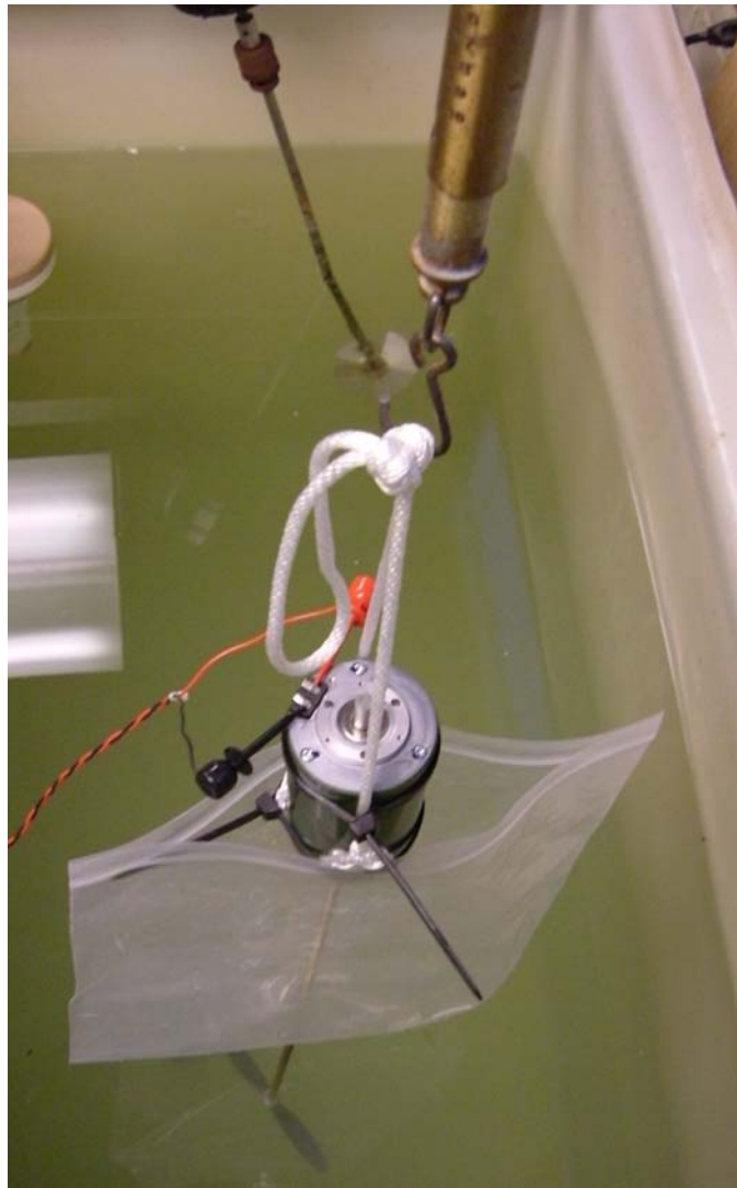
Photo 3: Propeller Testing Set-up
