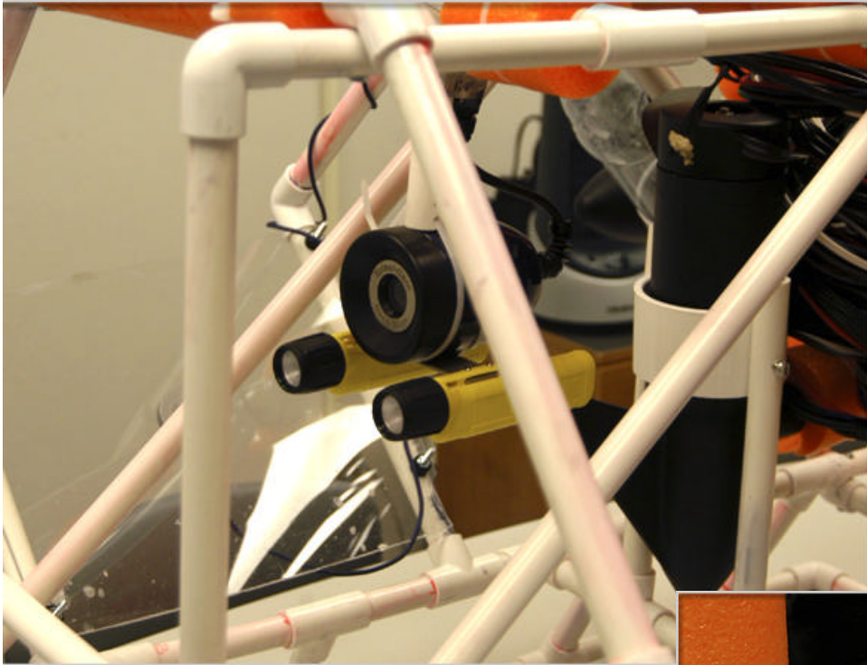
Picture 5. Freebie II ROV Deep Blue underwater Camera closeup
