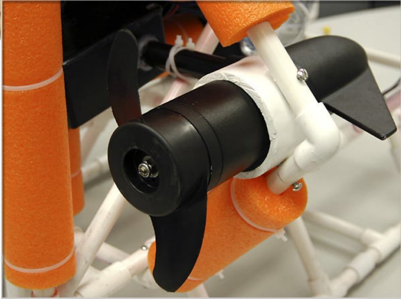
Picture 6. Freebie II ROV thruster (Minn Kota Endura 40 Trolling Motor)
