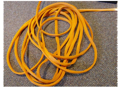
Fig 1.2 The tether; all wires leading from the submarine were fed through this orange sleeve along with polystyrene foam, coiled around the wires, for buoyancy.
