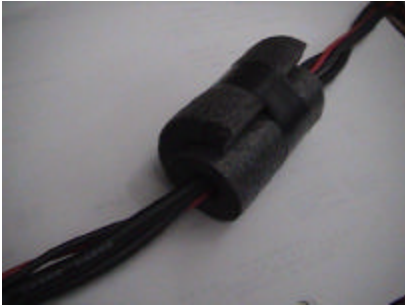
5.20 – Image of the Tether with buoyant foam
