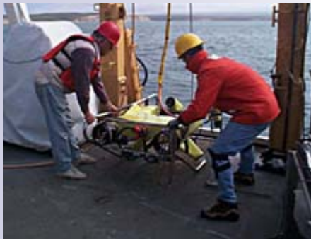
Remotely operated vehicles (ROVs) are essentially robots operated by a person aboard a surface vessel (Remotely 1)
