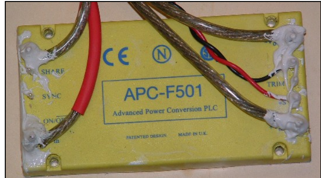
Figure 7 +48V to 24V 500W Power Supply
