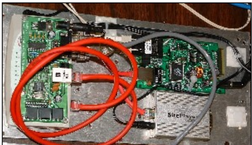
Figure 8 Ethernet Communications in ROV
