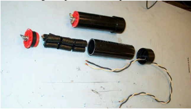
Figure 1.5 Batteries and battery pack
