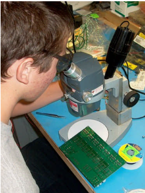
Figure 3.2 Nick soldering surface mount
