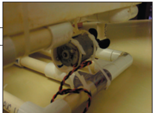
side motors and waterflow space
