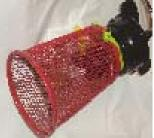
The two remaining bilge pumps are rated to move 3785 liters per hour and are used for vertical propulsion. These two motors, with the aide of the buoyancy system, create enough thrust to move the ROV vertically under the different loads required throughout the competition tasks.
