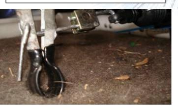
The newly made manipulator arm to grab instrument module box. Uses actuator from car doors.
