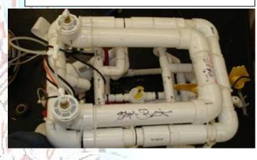
Top view. Notice the ballast tank (top ushaped). It is tied down by zip-ties.
