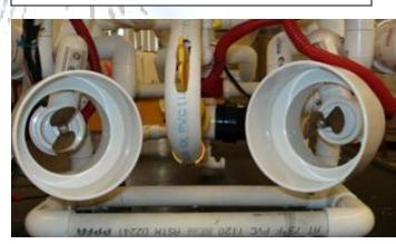
Angle mounted thrusters. Hard to see but are mounted inside the frame boundaries. Cowlings are also original. Might be disposed for weight issues.
