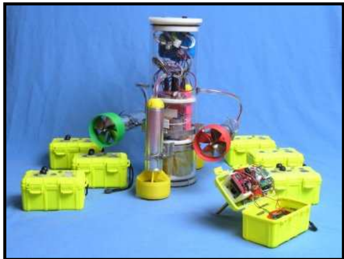
Several sensor nodes and AMOUR (Autonomous Modular Optical Underwater Robot) mobile node
