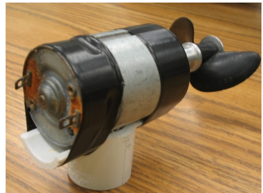
Figure 14. Rusty terminals on old motor
