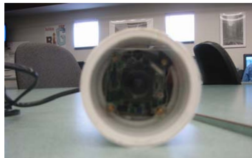
Figure 13: Close-up of camera inside casing
