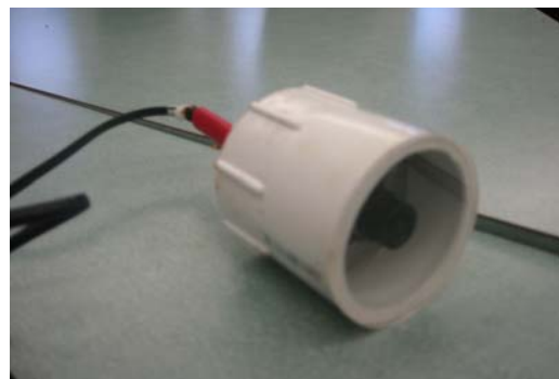
Figure 14: Casing around camera
