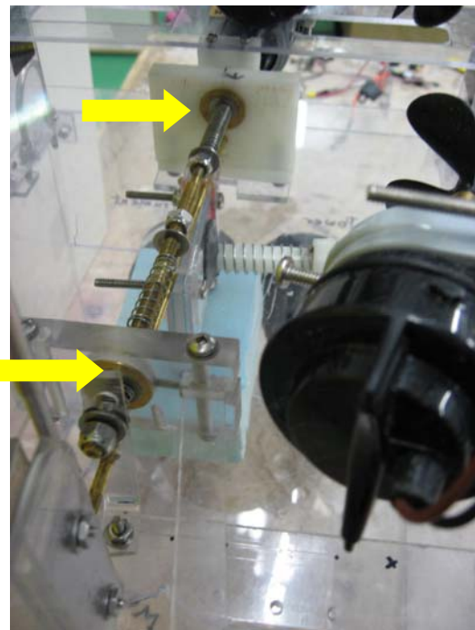
Threaded rod showing traveler plates for the front gripper and rear 'U'- bolt attachment sleeve
