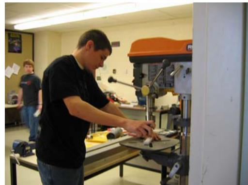
Drilling a hole into Lexan
