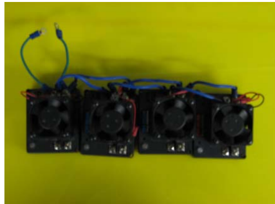
Victor 883 Pulse Width Modulators
