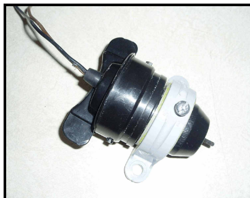
Figure 6. Bilge Pump Motor
