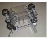
and held in place using straps. This configuration gives the ROV four degrees of freedom: heave, surge, sway, and yaw. This gives the ROV excellent control that makes it ideal for the complex underwater movement required. Polycarbonate is used for the frame because it is transparent, durable, easily worked, and very difficult to damage.
