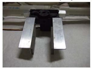
gripper mounted on the front of the vehicle. We are using just one gripper to both open the door and to pick up and carry the connectors to make things simpler. The jaw on the gripper opens in parallel to a width of over 2.5cm which is more than enough for both the <sup>1</sup>/<sub>2</sub>" PVC for the door and the U-bolt on the top of the
