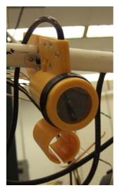
We are using a commercially available underwater camera. The camera is very similar to an X10 camera, but it comes manufactured with a built in lighting system and a waterproof housing using o-rings. Six white LEDs positioned around the camera lens comprise the manufactured lighting system. We modified the housing of the camera for mounting and, after examining the waterproofing, left it as it came.
