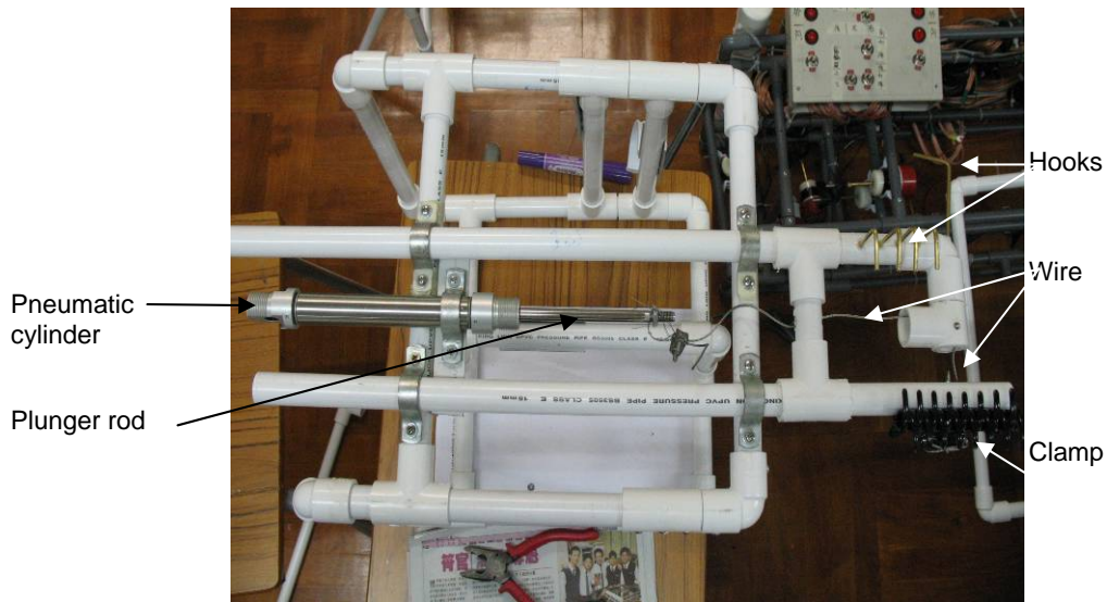
Photo 6: The pneumatic system and hooks on the small ROV ( bottom)
