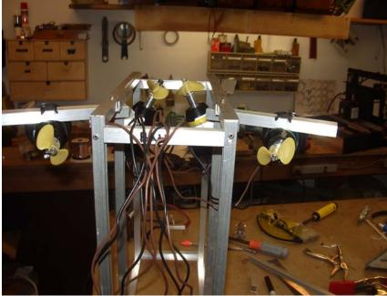
Figure 1.0: The two horizontal motors are positioned at a seventy-degree angle.
