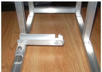
Figure 1.5: The manipulator centered at the bottom of the ROV.
