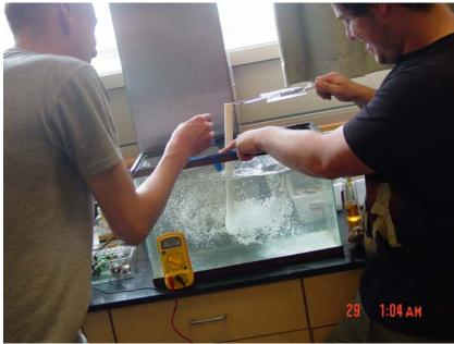
Figure 1.2: The motors being tested for thrust.
