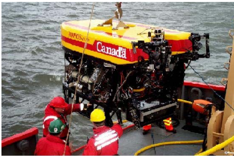
The Remotely Operated Platform for Ocean Sciences (ROPOS) getting prepared for launch at the VENUS node site. Image taken from University of Victoria. < http://www.venus.uvic.ca/gallery/index.html >
