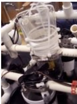
Figure 3-5: Vacuum to retrieve algae
