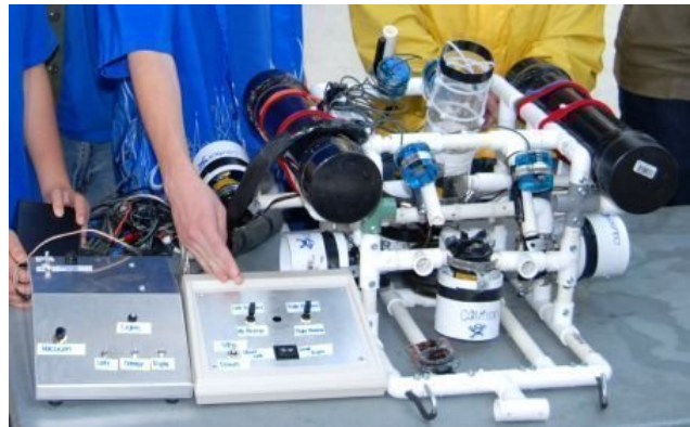
Figure 5-2: Original control boxes.
