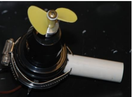
Figure 3-2: A bilge pump motor, fully assembled with mount, prop and adaptor
