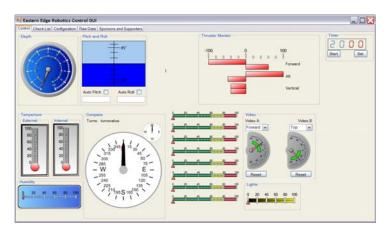
The Operations tab presents all data required for the ROV to operate. Some of the functions included are: a timer, camera tilt position, thruster power, tool position, power supply monitoring, humidity and temperature in the electronics can. An artificial horizon displays pitch and roll and provides a
