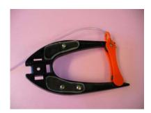
The tool for Mission 1 is an "off the shelf" mooring retriever modified to fit our ROV. A tool designed for this specific purpose is called the "Happy Hooker". It is a PVC I beam bent into a "U"-shape with a diameter of 15 cm. The opening of the "U" is blocked by a plastic bar, which is hinged on both ends. The "Happy Hooker" allows a line to pass through and return through the ballasted U-bolt. This tool can be fully detached from the ROV.
