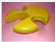
Flotation was constructed by laminating four (4) pieces of 50 mm thick H-100, low compression Dow Styrofoam Highload extruded polystyrene foam into a mass 200 mm deep, using an epoxy glue. This foam is ideal for the shallow depths of the competition as it is designed for use under extreme loads. It has a 692 kPa (100 psi) compression tolerance. The maximum
