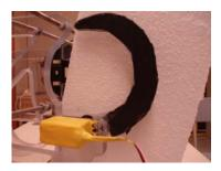
A multi-purpose "talon gripper" designed and fabricated for collecting the 'O'-ball, is located on the front of the ROV at its base. The "talon gripper" is fabricated using the 12.5 mm thick Lexan™ frame of the ROV as the fixed part of the claw and a 100 mm diameter curved arc of 6 mm thick Lexan™ forming the talon part of the claw. These parts intersect in a vertical plane. The talon part of the gripper moves in
