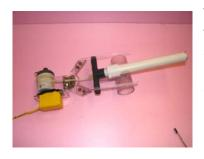
The tool used to inject the corrosion inhibitor is made from 6.0 mm thick Lexan<sup>™</sup> and uses a waterproofed servomotor winch directly connected to a spool to retract the line connected to the hot-stab. The hot-stab is inserted, the line is released and the ROV backs away from the wellhead. The hot-stab is retrieved when the injection is complete.
