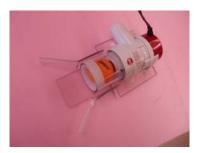
To collect a sample of algae, the ROV uses a bilge pump motor fixed at the end of 50mm Polycarbonate tube. When the ROV approaches the balls, the pilot turns on the bilge pump motor, creating a vacuum force, which sucks the balls into the tube. The balls are held in the tube by a ring of Velcro tape covering the inside of the tube.
