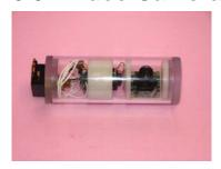
Bartlett uses three (3) high quality, low-light PC board cameras purchased from Super Circuits (PC169XS,) housed in clear 5cm O.D. polycarbonate tube with 3mm wall thickness. These color cameras have a 1/3" CCD with 460-line resolution and a 1.0 lux rating. They operate on 12 volts DC with low current rating of 110 mA. A 2.5 mm lens provides a 90° field of view in water. The cameras can be tilted (rotated 90°
