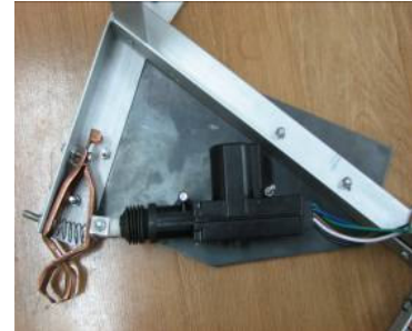
“Gripper made by car door lock actuator”
