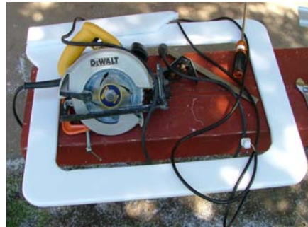
Figure 7: A cut frame side from HDPE
