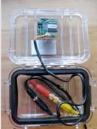
We attempted to seal our camera and connectors in a Pelican case. Unfortunately, the gasket admitted water. We then epoxied it shut, only to have the condensation inside the case short out the camera.
