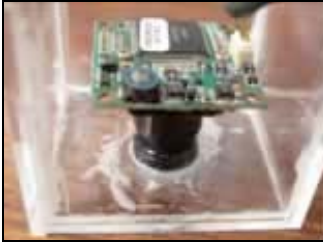
We built a plexiglass frame to house our board camera before encasing it in epoxy.
