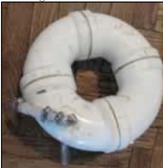
The “doughnut” was our first attempt at making a variable buoyancy system, which we hope to improve and include in next year’s ROV.
