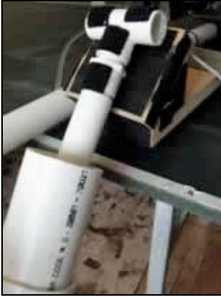
The hot stab grabber demonstrating the insertion of the hot stab into the wellhead.
