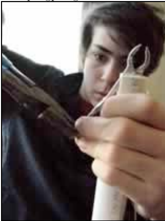
Joshua fabricating the hydraulic syringe system for the alligator clip hand.
