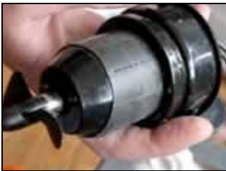
We covered the thrusters with bicycle inner tubes so that they would fit snugly into the mounting hardware.
