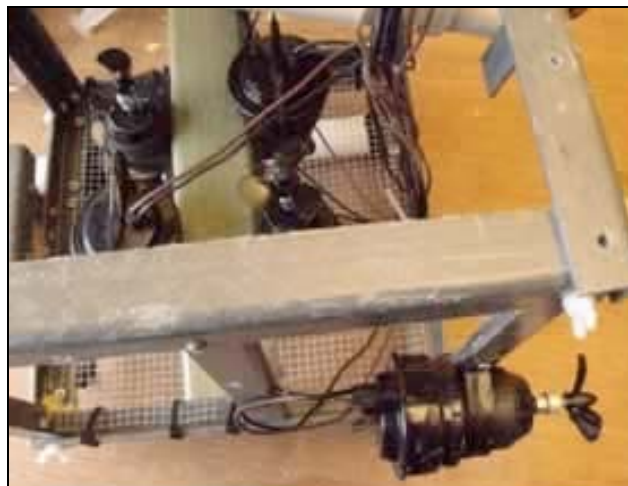
This shows our thruster mounting system prior to installing propeller shielding. The holes and cuts in the frame indicate where things were attached previously in different incarnations of Proto's life.
