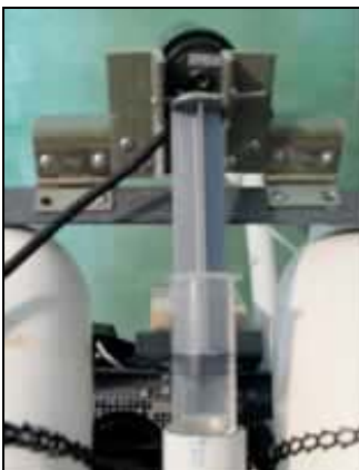
This rear view of the camera tilt system shows the syringe attached to a hinged piece of angle on which the camera is mounted. This enables our camera to tilt almost 180 degrees.
