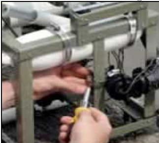
After testing in Hudson River currents, we added two more forward/reverse thrusters.
