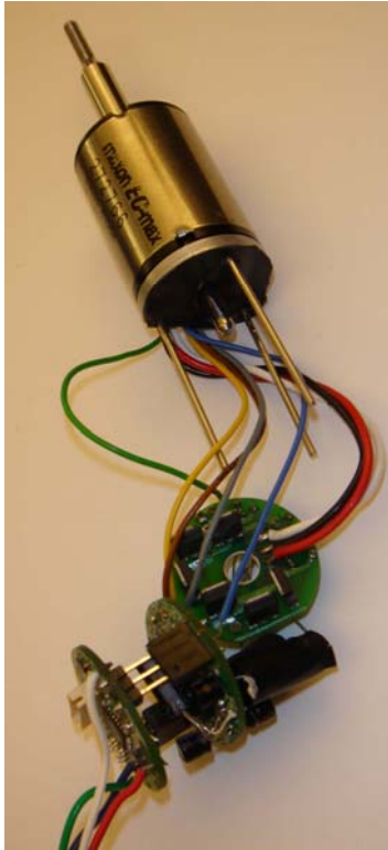
Figure 17 – Custom Motor Controllers
