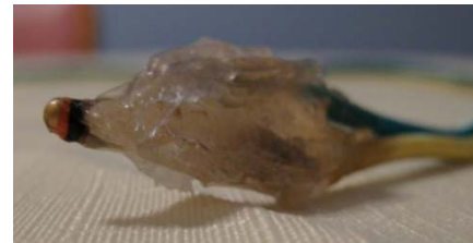
Fig. 3.5 The thermistor after waterproofing
