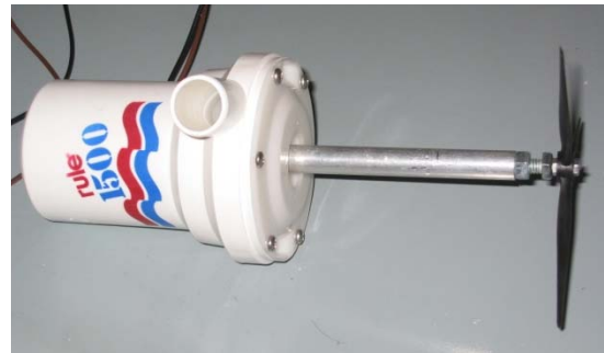
Fig. 3.2 A complete motor assembly with a custom adaptor and a propeller
