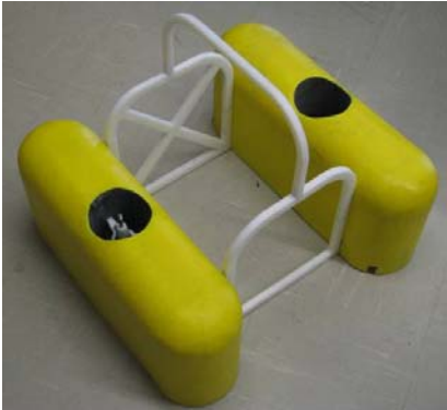
Figure 2. pontoons with HDPE frames
