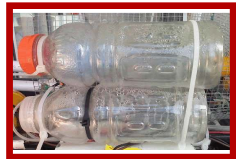
Figure 10: Buoyancy System of Stacked Gatorade Bottles
