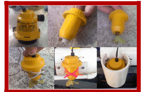
Figure 9: Development of a Thruster from a Bilge Pump
