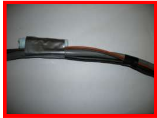
Figure 4: Tether showing extra motor wire, buoyancy, temperature sensor, and camera wire.
