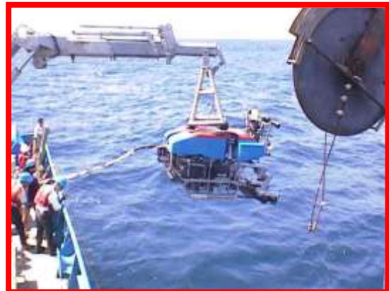
Figure 19. Jason vehicle being launched from RV Atlantis in the Guaymas Basin, Sea of Cortez. 4
