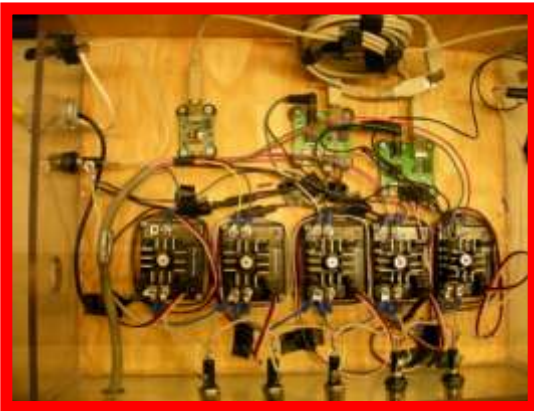
Figure 2: Phidgets and electronic speed controllers in control box
