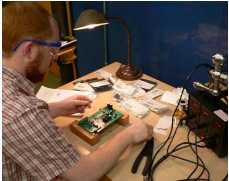
Figure 14 - Adam Works on Soldering the Control Board
