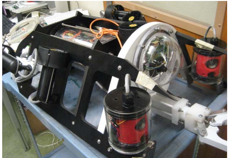
Figure 16 - ROV in Position for Programming Updates
