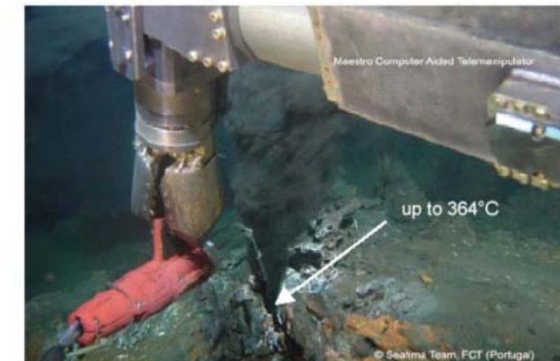
Fig. 7: Seahma-I (2002) cruise: Maestro manipulator operator is performing precise temperature measurements in a black smoker (Rainbow hydrothermal field, venting temperature up to 364°C).
