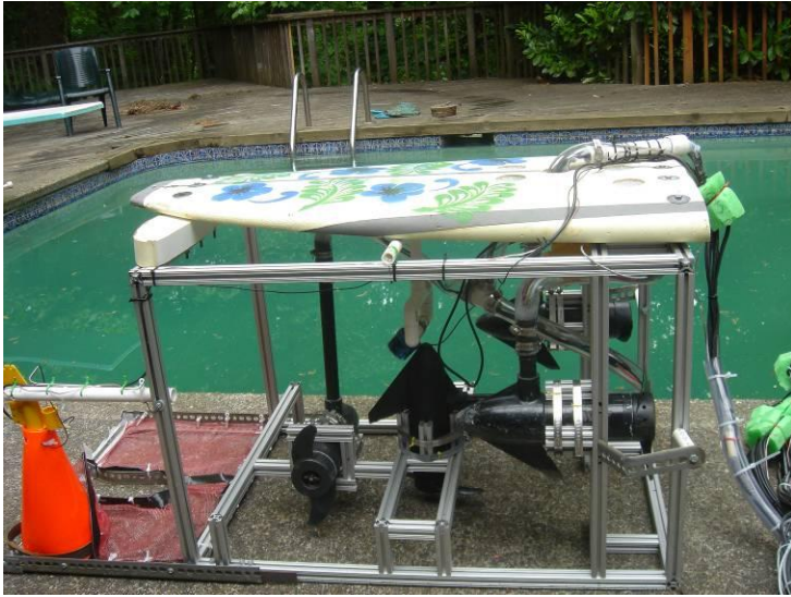
Side view of ROV illustrating the layout of our thrusters
