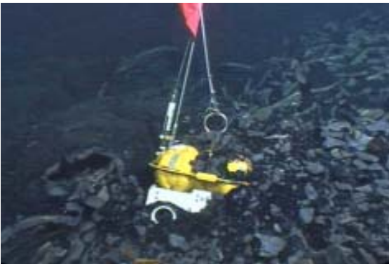
Figure 8.2 An OBS trapped in lava flow (Photo courtesy of http://www.whoi.edu/oceanus/viewArticle.do?id=27286 )
