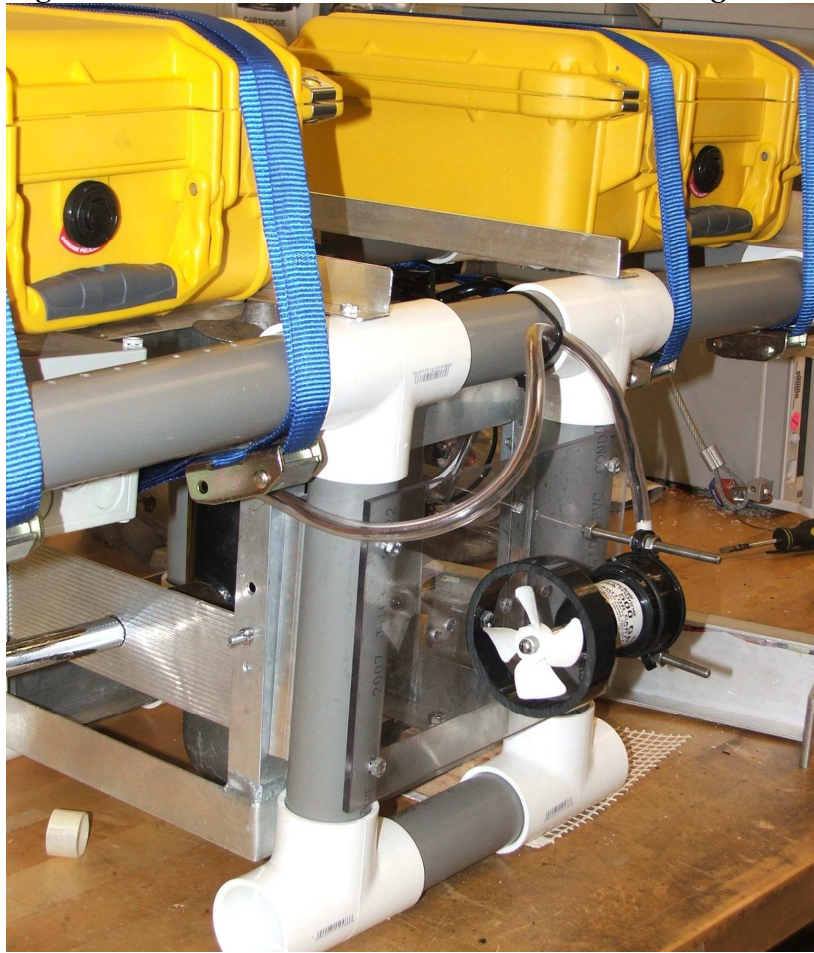
Figure 6a&b: Side thruster with shroud on Sea-Slug frame
