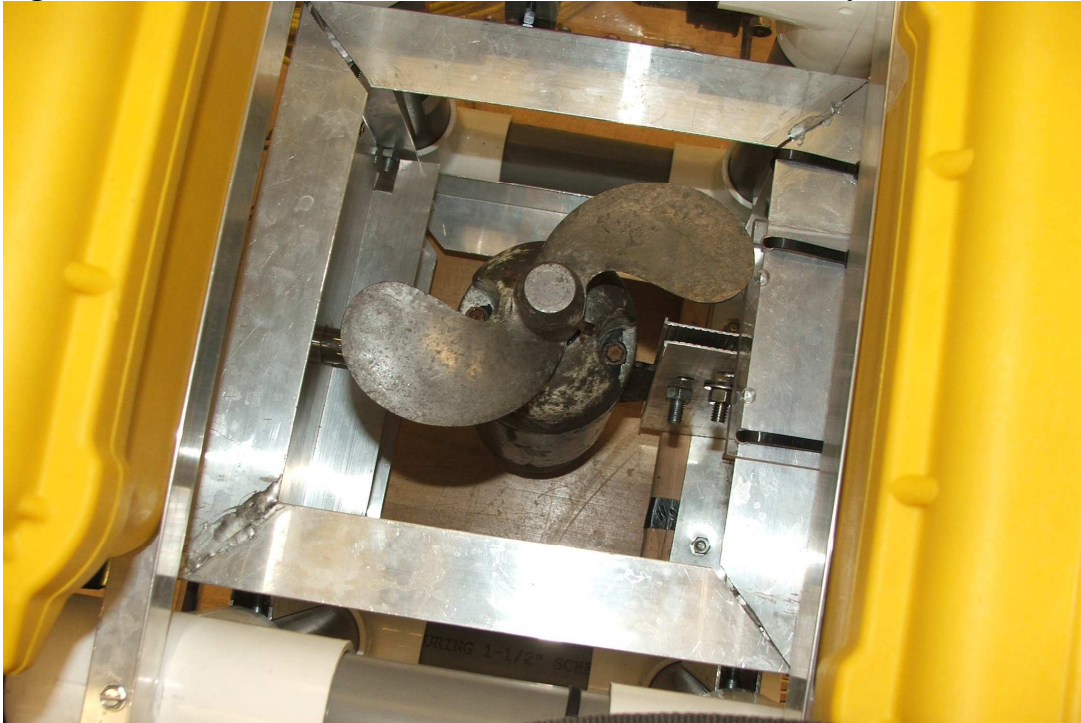
Figure 7: Aluminum frame for vertical thruster surrounded by floatation cases.
