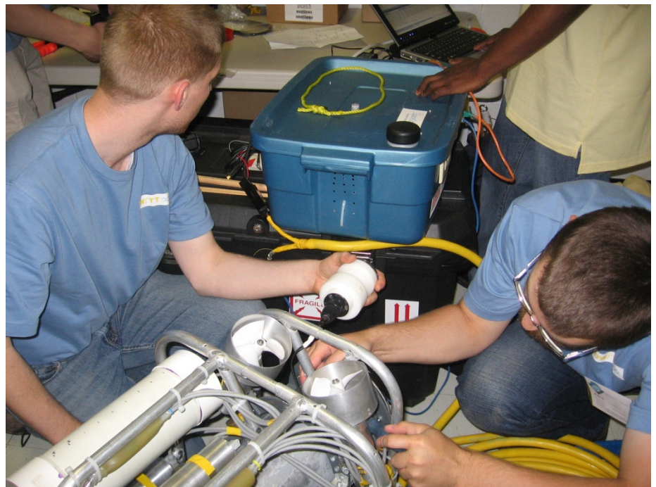
Repairing the ROV, View of ISD and Control Box
