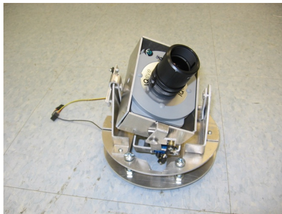
Figure 3: Camera Mounted in Pan and Tilt Mechanism
