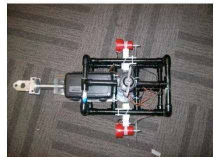
Final Aquabot frame with complete thrusters and arm
