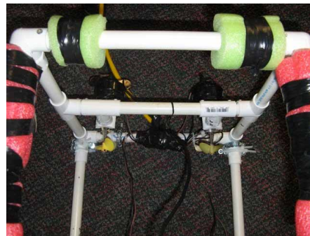
Figure 13: Back of the ROV frame, floatation, two thrusters, part of the tether, and ballast on the bottom.
