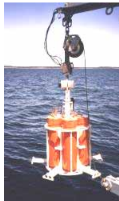
Figure 20: Close-up view of ELSS pods before they are launched by the LARS
