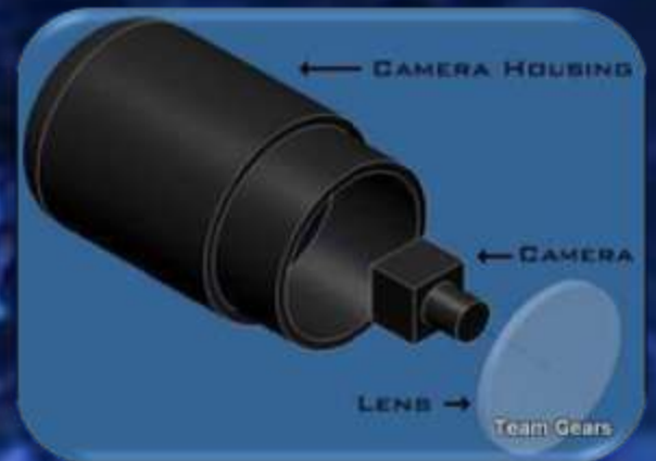
(Figure 20) Our water proof camera is incased in a protective PVC housing
