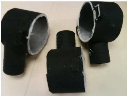
Bilge pump casings used as camera mounts
