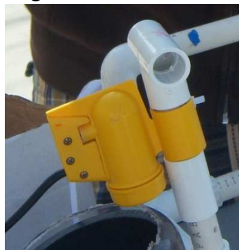
Camera for the transfer skirt
