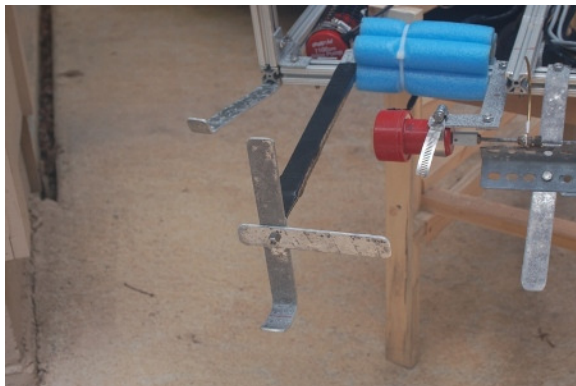
Figure 11: Pod Hook (left) and Manipulating Hook (right)
