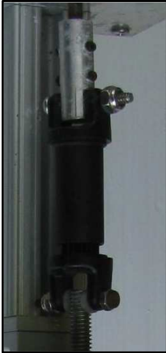
Image 10: The axel connecting the gear box to the gripper system with the new stainless steel screws replacing the cotter pins was much more reliable
