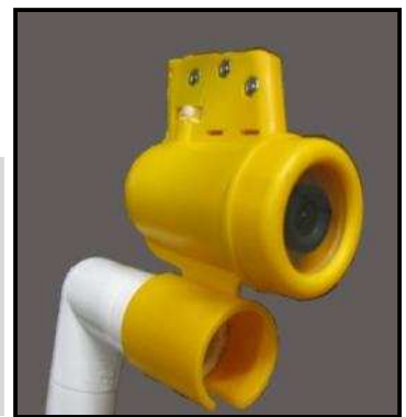
Image 8: One of the six cameras used to monitor and operate the ROV. Cameras were essential to the ROV.
