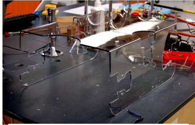
Figure 3 Lexan frame prior to mounting components.
