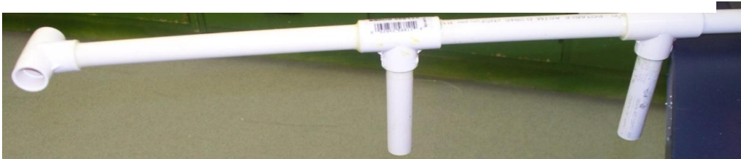
Figure 13 1/2" PVC pipe arm
