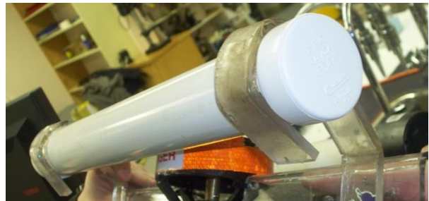
Figure 9 PVC pipe for flotation
