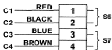
RIGHT SIDE TERMINAL BLOCK
