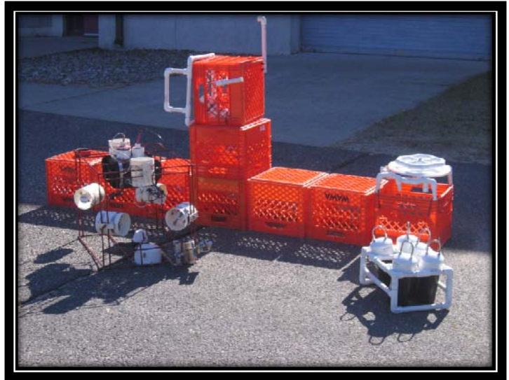
Figure 3: View of ROV (front left) with Submarine (back) and Pods (front right)
