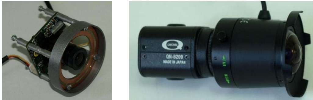
Fig. 5. Video cameras: a) survey and rotatable; b) navigational
