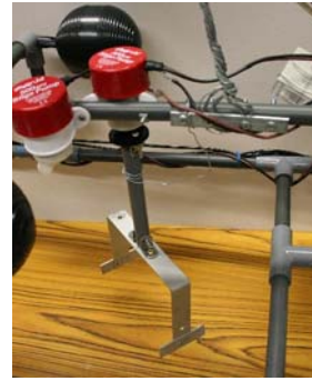
Robotic arm made of aluminium for turning the escape hatch
