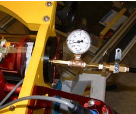
FIGURE 22 – VACUUM LEAK TEST SETUP
