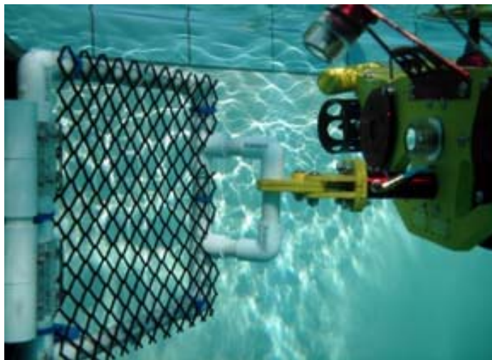
FIGURE 2 – SPEAR OPENING AIRVALVE ACCESS HATCH FOR TASK #3
