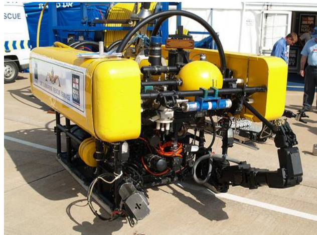
Figure 11: Scorpio 45, ROV of the UK Sub Rescue Service 6
