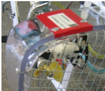
Fig. 11: A view of one side motor and its protection.
