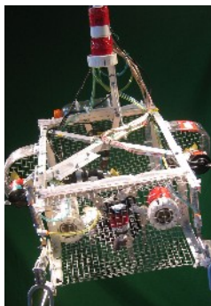
Fig. 4: The finished frame, with the cross-pieces visible.
