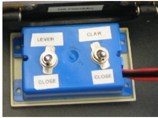
Fig. 10: The pneumatic switch box.
