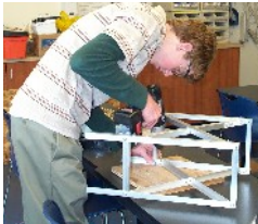
Fig. 2: David Lundberg constructs the original ROV frame.
