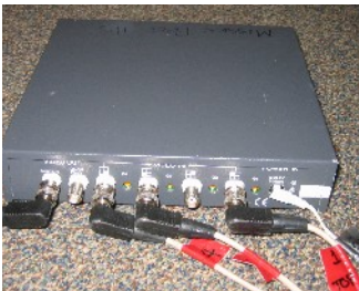
Fig. 6: The quad-splitter allows us to view all three cameras on a single TV at once.
