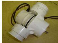
Figure 5: Customized PVC piece for motor
