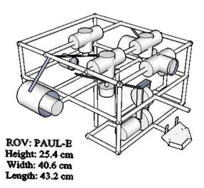
Figure 2: Final CAD Model
