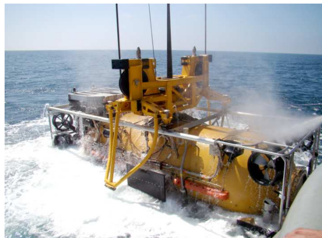
Figure 15 - PRM Module being recovered from rescue exercise (Courtesy of Navy.mil)
