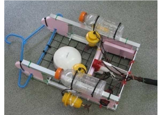
Figure 9 - ROV Osprey with two Gatorade bottles
